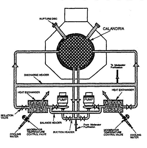
Relief valves, connected to the cover gas system provide overpressure protection to the moderator system and the calandria during normal plant operation.
